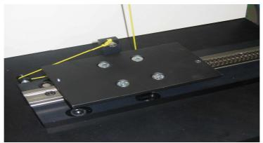
3° Mount the Upper Fixture (AC PINCE – mini wedge) to the load cell stud and tighten.
